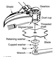
**NOTE:** Make sure all parts are in place as illustrated, and the blade is sandwiched between the dust cup and the retaining washer. There should be no space between the blade and the dust cup or the retaining washer.
